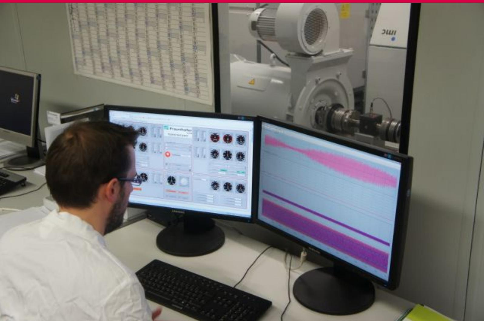
Optimized powertrain topology and design are essential for achieving progressive development of electric vehicles. On behalf of the Fraunhofer Institute (IFAM Bremen), imc Meßsysteme GmbH has developed a test station with two testing tracks and an integrated simulation solution, enabling the development and testing of new components for and models of electric motor powertrains.
